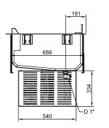
D = Drain EI = Electrical inlet (power)
